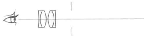
Plössl (Pl) Georg Simon Plössl, 1860 Improved by Nagler, 1979 Apparent field 50° Eye relief 80% of focal length
