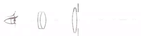
Kellner (K) Achromatic Ramsden (AR) Modified Achromatic (MA) Carl Kellner, 1849 Apparent field 40° Eye relief 40% to 50% of focal length
